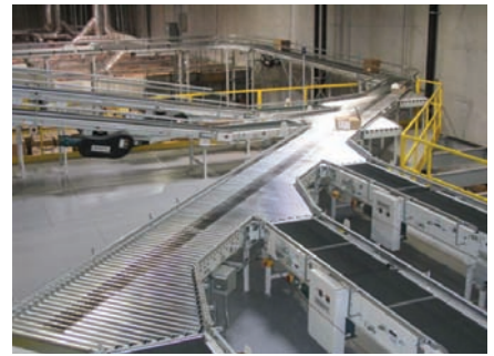
The sortation system sends packages to a shipping area, where cartons will be staged for delivery.
